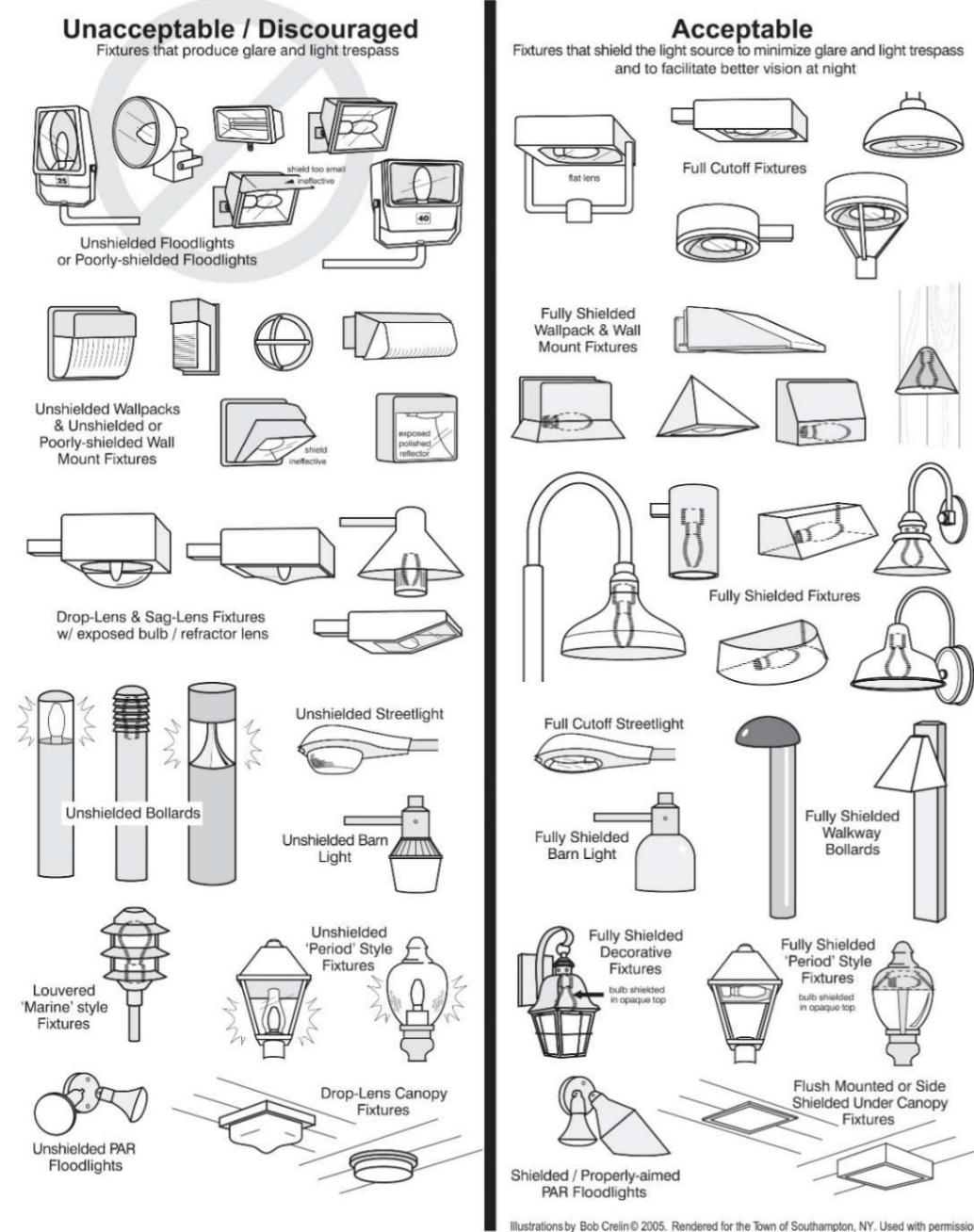
Figure 4—1 Example of luminaire types approved by the IDA - (Source IDA)
