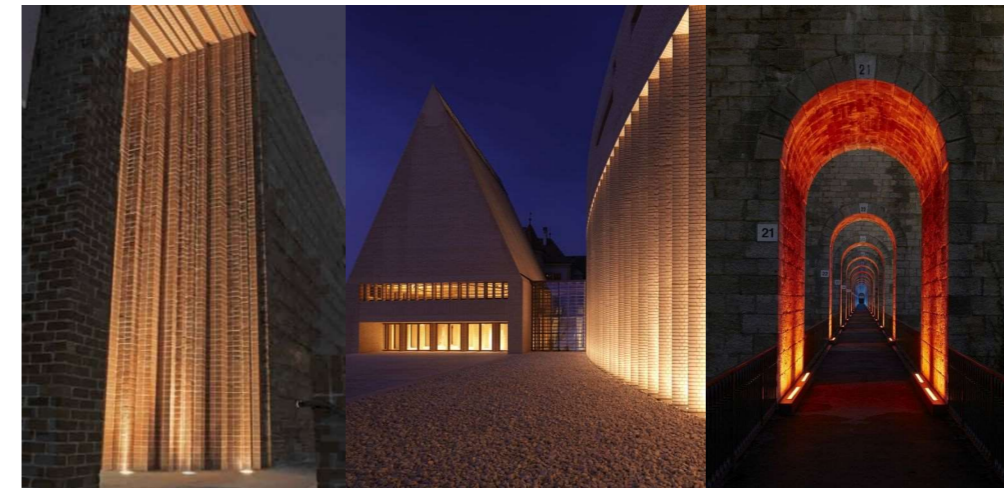
Figure 6—26 Precedent image of inground luminaires used to highlight access points or gateways
